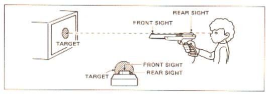
Point the ZAPPER toward the target and aim so that the target, the front sight, and the rear sight are all aligned.
